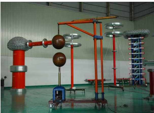
Test room 250 kV apply Voltage and 1800kV impulse voltage generating equipment
