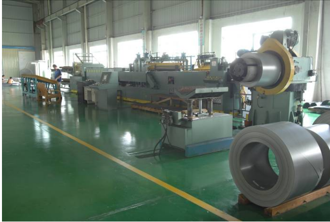
Step-lap cover cutting machine with automatic stacking functions
